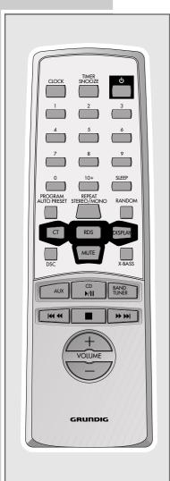
U Switches the stereo system to and from stand-by mode.
